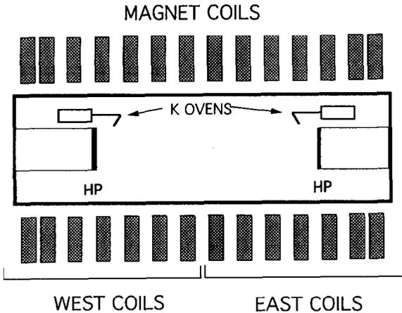
Fig. 1. Schematic diagram of the double-ended Q machine. The west and east magnet coil sets can be powered independently to produce various magnetic field configurations.
