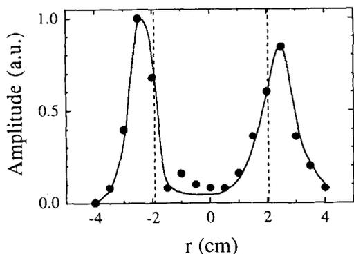
Fig. 3. Oscillation amplitude versus radial coordinate,  $r$ . The dotted lines correspond to those in Fig. 2. The maximum fluctuation amplitude corresponds to a  $\delta n/n \approx e\delta\phi/kT_e \approx 0.7$ .  $I_W = 900$  A,  $I_E = 200$  A.
