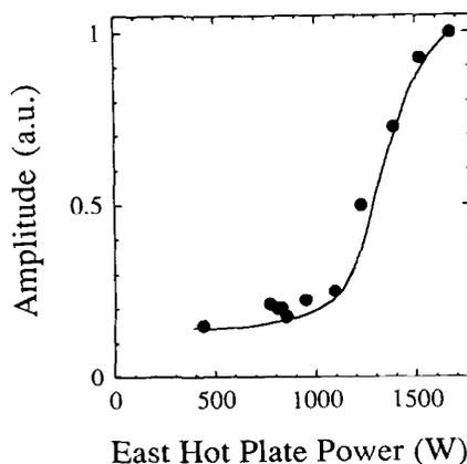
Fig. 5. Dependence of the oscillation amplitude on the east hot plate power.  $I_W = 900$  A,  $I_E = 200$  A.
