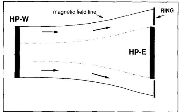
Fig. 2. Schematic diagram of the double-ended Q machine with a diverging magnetic field configuration. The solid lines represent field lines mapping from the edge of the west hot plate (HP-W) and the dotted lines those from the east hot plate (HP-E). A non-flowing plasma is produced in the region between the dotted lines, while a plasma flowing from west to east is produced in the outer region and is terminated on the floating ring.
