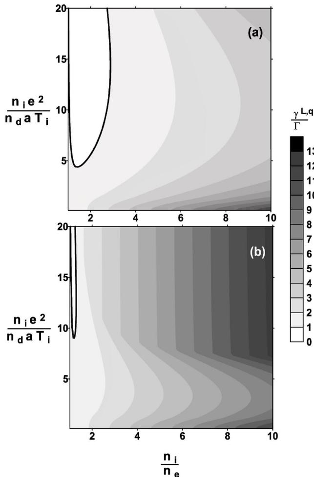
FIG. 2. Relief of the ratio  $\gamma_k^{L,q}/\Gamma$  on the plane  $(n_i e^2/n_d a T_i, n_i/n_e)$  for the plasma parameters (a) in the experiments of Ref. 14 and (b) in the experiments of Ref. 13. The heavy curves correspond to  $\gamma_k^{L,q}=\Gamma$ .
