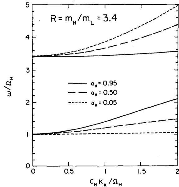
Fig. 3. Dispersion relation for EIC modes in a two-ion plasma with mass ratio 3.4 for various values of the heavy-ion concentration  $\alpha_H = 1 - \alpha_L$ .
