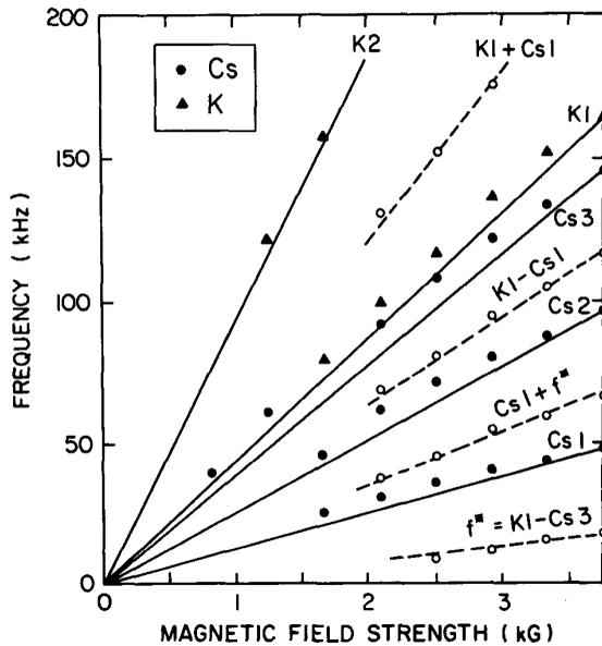
Fig. 2. Frequencies of EIC modes as a function of the magnetic field strength. The solid lines are the  $\text{Cs}^+$  and  $\text{K}^+$  EIC harmonics. The dashed lines indicate sum and difference modes.
