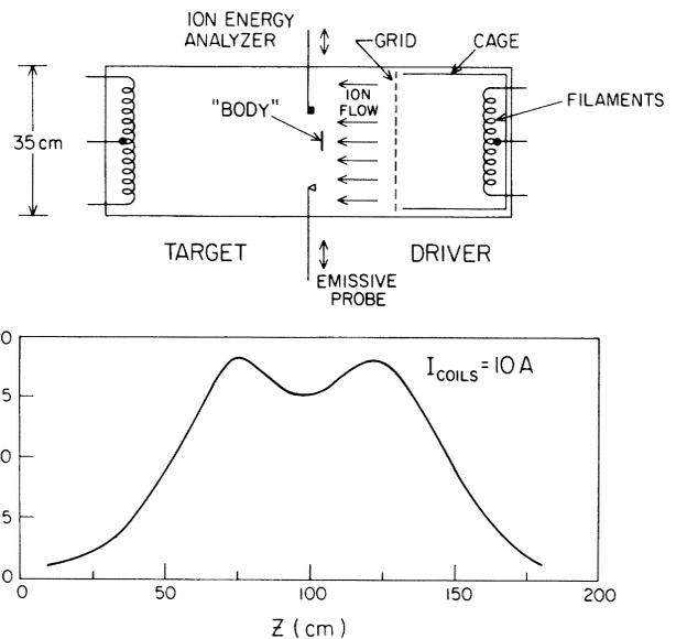
Fig. 1. Schematic of the experimental setup. The profile of the axial magnetic field for a coil current of 10 A is also shown, on the same scale.
