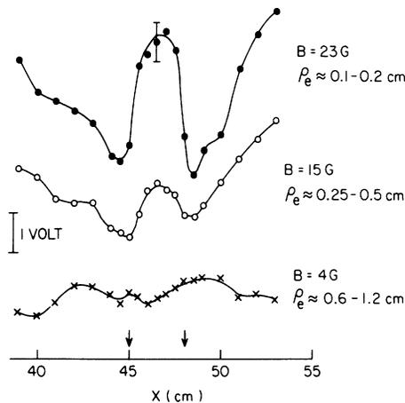
Fig. 3. Potential profiles in the body wake in a direction transverse to the ion flow, for several magnetic field strengths. The corresponding electron gyroradii are also shown. In each case the ion gyroradius is much larger than the transverse body dimension. The vertical arrows indicate the edges of the body. For clarity, the plots are displaced vertically.
