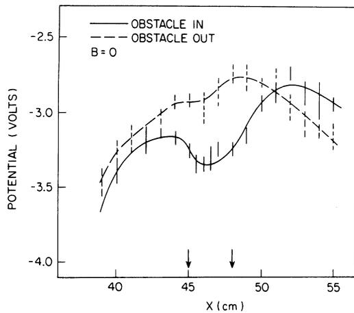
Fig. 2. Potential profile (full line) in the body wake in a direction transverse to the ion flow.  $B = 0$  G. The vertical arrows indicate the edges of the body. The dashed line was obtained with the body removed.
